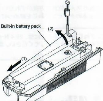
7. Place a new built-in battery pack properly inside the display unit.
