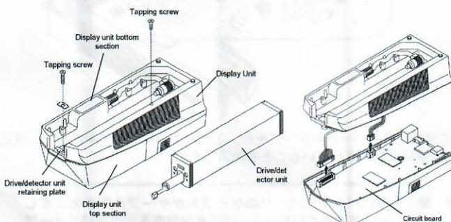
5. Detach the cable of the built-in battery pack from the cable support plate.
