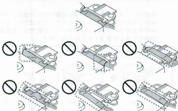
10. Reconnect the connector, which connects the top and bottom sections of the display unit, and built-in battery pack connector to the board in the display unit.
