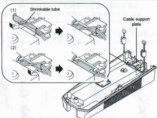
9. Check that the cable of built-in battery pack is fastened and are wired securely as shown below.
