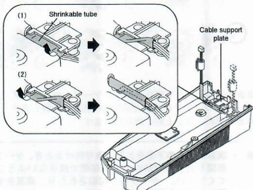
6. Remove the built-in battery pack from the display unit.
