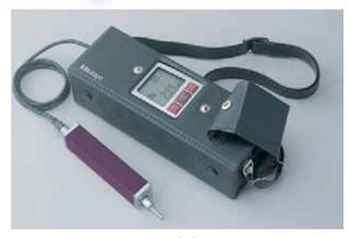
The built-in battery if fully charged allows approximately 500 measurements to be taken even on a site with no access to power.
