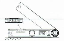
\* Place fixed blade on the measured surface. If the bubble inside the vial stays between the marks on the vial's surface, the measured surface is horizontal.
