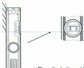
\* Place the bottom side of fixed blade tightly on the measured surface. If the bubble inside the vial stays between the marks on the vial's surface, the measured surface is vertical.
